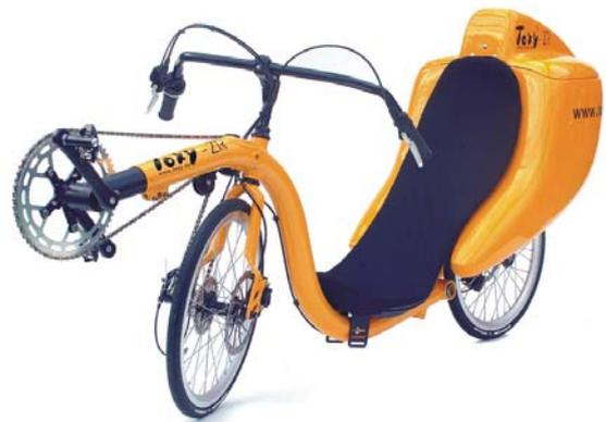
**The ultimate star** of this year’s Toxy-Show was the updated Toxy-ZR, assembled as an ultra-tourer with its optimized Rohloff Speed-hub front wheel drive, the lockable, aerodynamic luggage bag, and a prototype of the latest Schmidt single sided generator hub at the unique rear monolever.
