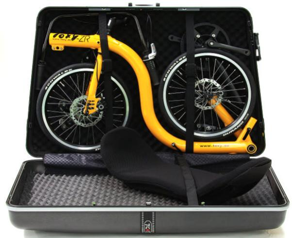
The new Toxy-ZR „RaceCase“ comes with a longer mono rear lever, which allows to fold the rear wheel into the main frame. So it is possible to pack the complete ZR into the rigid Race-Case, including the seat and all components. – Furthermore there is enough space left for your race clothing, bicycle shoes and other equipment.
